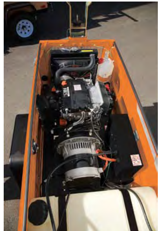
Engine and components are easily accessible with top panel up. Crossbar can be removed and side doors can be opened with panel raised.
